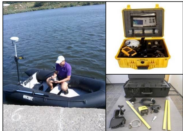
Figure 3.24. Used instruments and mounting method on an inflatable boat
