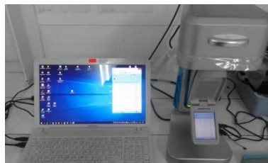
Figura 2.23. Spectrometrul ED-XRF, Genius 5000, Sky Instruments
