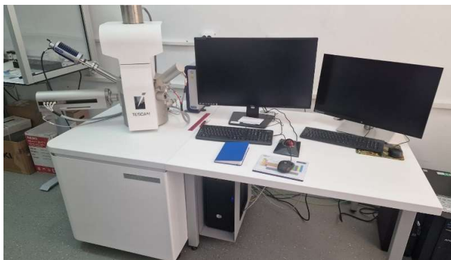
Figura 3.2 a Echipament SEM TESCAN VEGA (foto Georgiana Ghisman)
